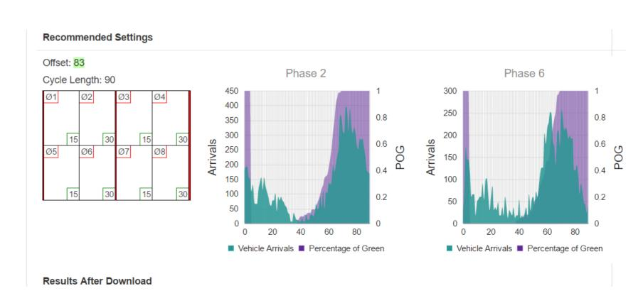
Update phase 2&6 split times to 22 seconds and 4&8 to 15 seconds to reduce split failures
