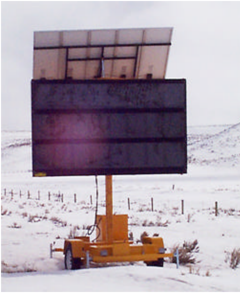
Figure 2: Portable Dynamic Message Sign (DMS) in Idaho.
